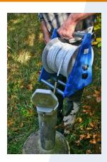
Water level meters are part of the standard equipment for the ascertainment of ground water levels. These mobile units are characterised by their simple, fast and solid acquiring of water level. With the variety of available models, you have the possibility to select the appropriate unit according to your individual requirements in cable length or operating convenience.
