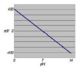
Figure 1. pH sensor calibration graph
