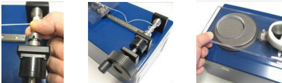
Fig. 6: Quick adjustment of the winding mechanism for placement into furthest left position.
