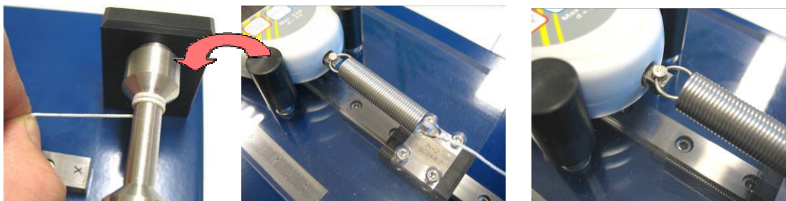
Fig. 7: Quick winding the first part of the cord; be sure the spring is in the horizontal position.
