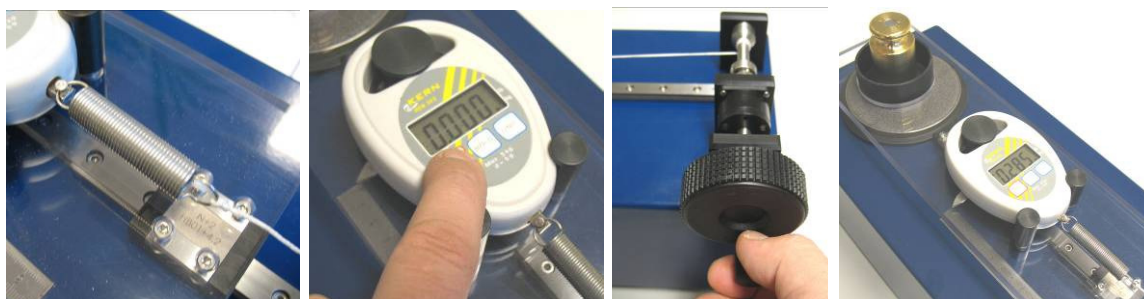
Fig. 15: Tare the scale, start winding smoothly clockwise, reading the maximum value after minor movement.
