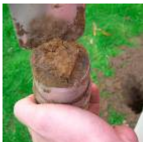
Figure 29: Chip off excess soil – don't smear!
