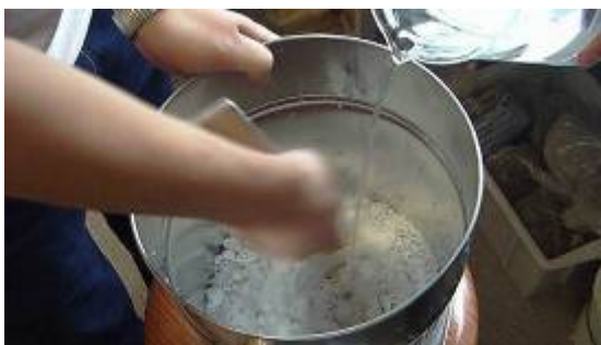
Figure 16: Saturate sand with water
