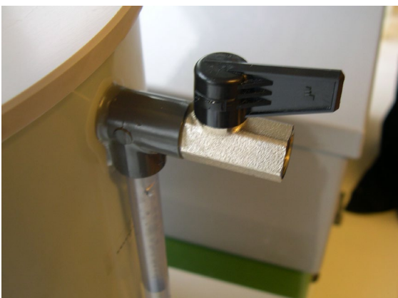
Figure 44: Open the pressure release valve
