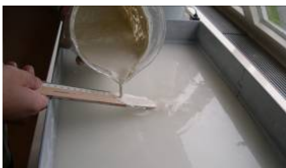
Figure 18: adding the water-saturate sand
