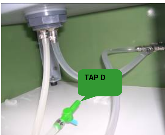
Figure 10 : TAP D at backside of the box
