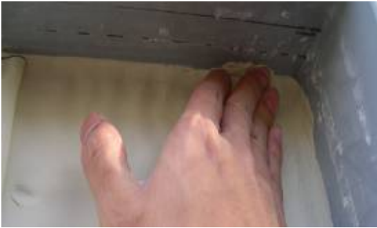
Figure 25 : Press the kaolin against the walls
