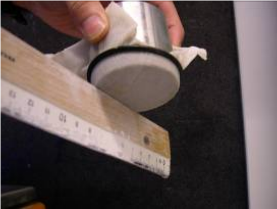
Figure 39 : Smoothen the extra water on the sample
