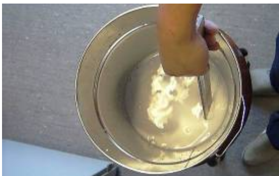
Figure 17: A high ratio of water to sand
