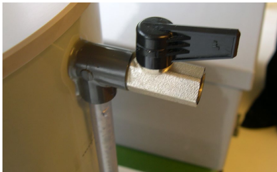
Figure 12: Open the pressure release valve
