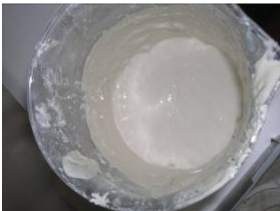
Figure 22: Water-saturated Kaolin clay
