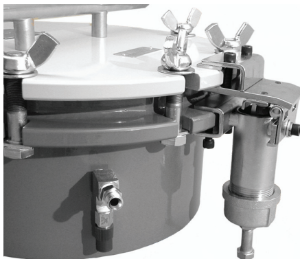
Fig. 6 - Protector Cap on Pressure Inlet Fitting
