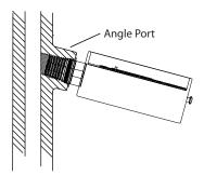
(Fig. 5) Attaching the dial gauge
