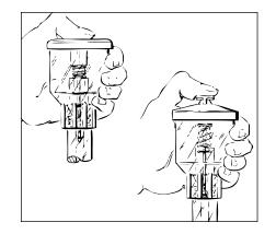
(Fig. 7b) Removing the air from the Tensiometer Body
