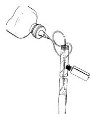
(Fig. 6) Filling the Tensiometer
