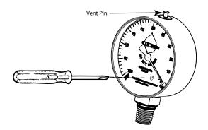
(Fig. 3) Vacuum Gauge Adjustments
