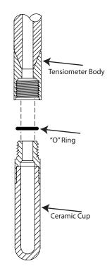
(Fig. 4) Attaching the Ceramic Tip
