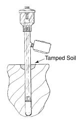
accept the tensiometer are always backfilled and the soil at the surface tamped tightly around the body tube. (*Fig. 8b*)
