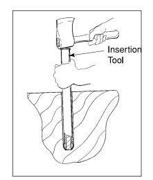
(Fig. 8a) Coring the hole
