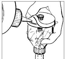
(Fig. 7a) Filling the Jet Fill Tensiometer
