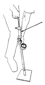
(Fig. 6a) Pulling a vacuum inside the Tensiometer using the Vacuum Hand Pump.
