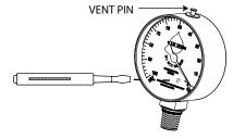
(Figure 4) - Venting the gauge
