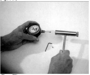
Fig. 32 shows the dial gauge removed from the handle. The internal connecting tube usually remains in the dial gauge. Carefully pull out the internal connecting tube from the dial gauge.
