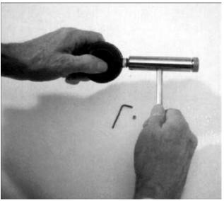
Then grasp the dial gauge firmly, as shown in Fig. 31, and turn it counterclockwise until it is free from the handle.
