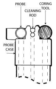
(Figure 3) - Probe case Tool placement
