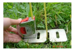
The reading on the measuring tape  $(Y_0)$  is immediately recorded and a stopwatch activated  $(t_0)$ .
