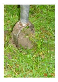
You may tap the auger body on the ground to remove the soil. Sticky soil should be removed by hand.
