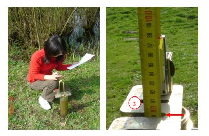
Remove float and measuring tape and bail out the water using the stainless steel bailer connected to the upper part and/or extension rod.
