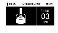
The measurement starts automatically after the end of the reaction time.
