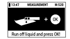
Carefully allow excess liquid to run off via the long edge of the strip onto an absorbent paper towel and press the [OK] button.
