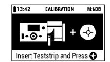
Insert the calibration strip of the recalibration set (included in the scope of delivery of RQflex® 20) into the strip adapter with the beveled edge outwards and upwards and press the [START measurement] button.
