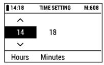
Select the desired time using the [Up] and [Down] buttons.
