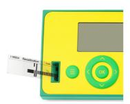
Make sure that no test strip ist inserted in the test strip adapter, then press [OK].
