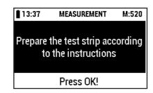
Immerse the test strip into the sample as described in the Reflectoquant® package insert (Reflectoquant® pack) and press the [OK] button.
