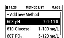
Select the desired method using the [Up] and [Down] buttons.
