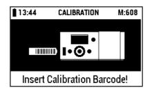
Remove the barcode strip for calibration from the pack (included in the scope of delivery of RQflex® 20).
