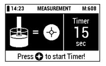
Immerse the test strip into the sample as described in the Reflectoquant® package insert (Reflectoquant® pack) and **at the same time** press the [START measurement] button to start the timer.
