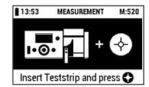
Insert the test strip into the test strip adapter and press the [START measurement] button.
