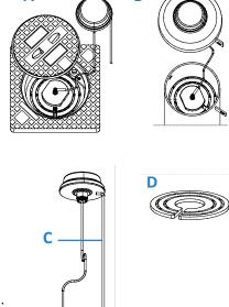
Adjust the universal monitoring well adapter ring (D) to your monitoring well so that the modem hangs correctly in the monitoring well. Then connect the sensor cable to the modem. Install sensor, sensor cable and modem into the well cover.
