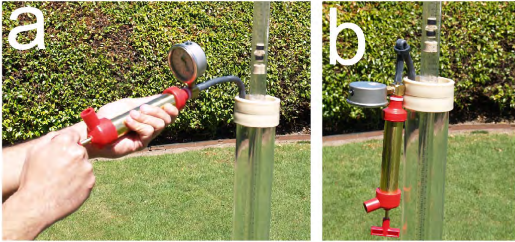
Fig. 36. Applying vacuum to Reservoir.
