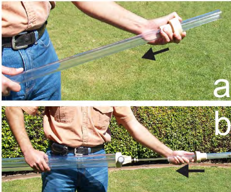
Fig. 23. Assembling the Tripod Bushing and Support Tube.
