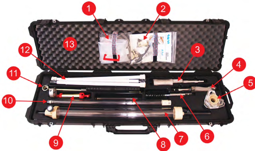
Fig. 5. Guelph Permeameter Kit (2800K1) components in Carrying Case.
