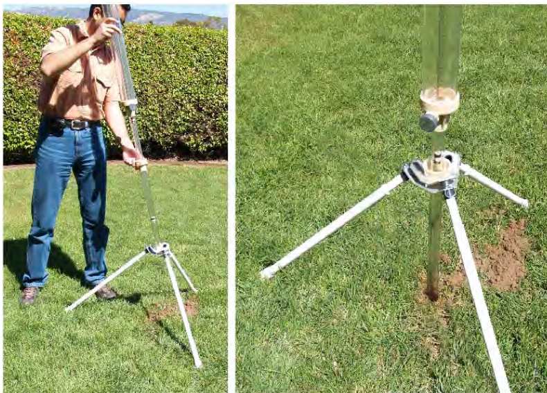
Fig. 24. Left: lowering GP into Tripod and Borehole. Right: GP is stabilized by pushing the Tripod Bushing into Tripod Base.
