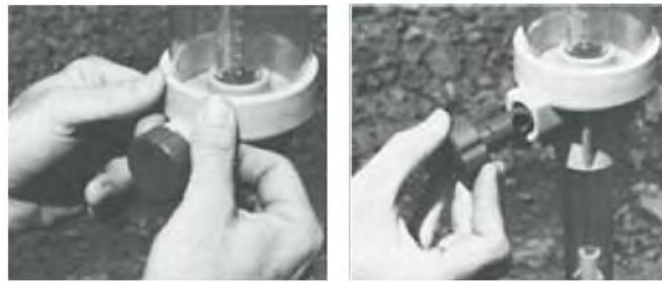
Fig. 37. Removing Reservoir Valve.
