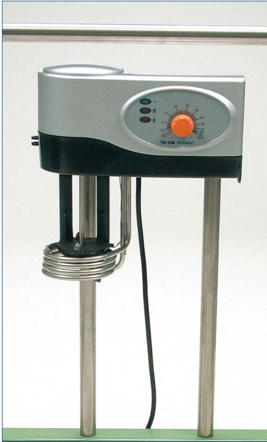
Figure 3 Installation of the heating element
