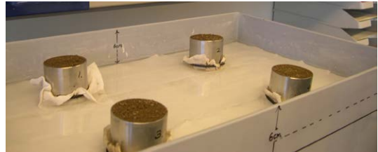
Fig. 32 Allow samples to adapt for 1 hour
