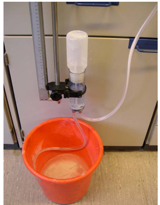
Fig. 15 Suction regulator at maximum
