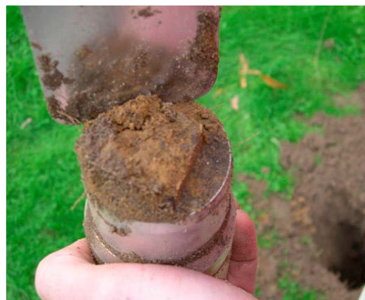
Fig. 29 Chip off excess soil - don't smear!
