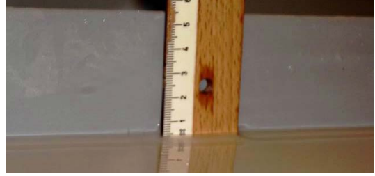
Fig. 31 Retain 0.5 cm water above the sand
