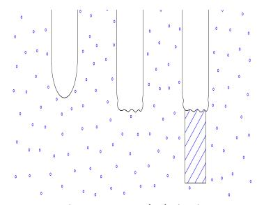
Auger hole with Edelman auger (left), Riverside auger (middle) and root auger (right)
