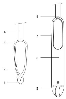
Edelman auger combination type (left) and Riverside auger (right).
