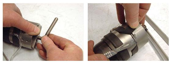
Push the ring with clamping pins over the cutting ring and fit the new nuts that are included in the set by hand. Tighten the nuts **alternately and a little further each time** using the box spanner. After that, you can remove the clamping tool and fit the cutting head back into the frame.
