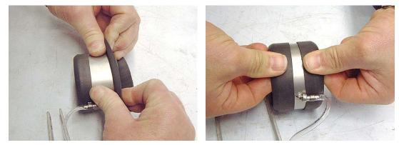
Extra requirements: New cutting ring (if old one is damaged), clamping tool.
