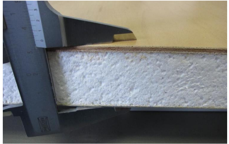
Example sandwich: aluminum - insulation - plywood
