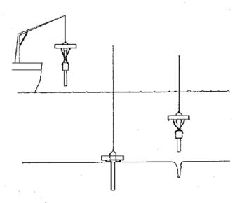
Fig.2 Use of the free-fall corer
