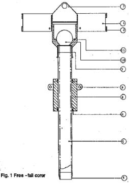
transparent sampling tube (5). The falling weight (8) hangs on the frame with chains through ears (9); a rubber bush (6) secures correct leading. A rubber ball valve (10) in the valve house (11) keeps the sample in the tube through vacuum.
