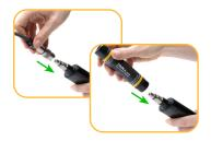
Align the flat edge of the connector with the flat edge inside the cable.
