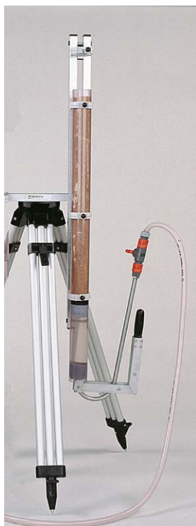
Discharge and partitioning system (04.23.SB set)
