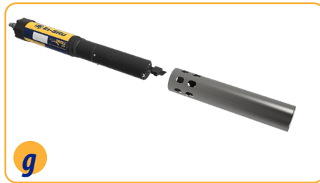
Flip restrictor and install with restrictor holes near center of instrument for calibration.
