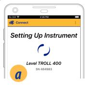
Attach an instrument and turn on the Wireless Rugged TROLL Com. Launch VuSitu. The app will automatically connect.
