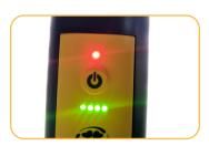
The device lights will turn on and blink according to charge level.
