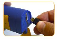
Disconnect the Wireless TROLL Com from a power/charging source.
