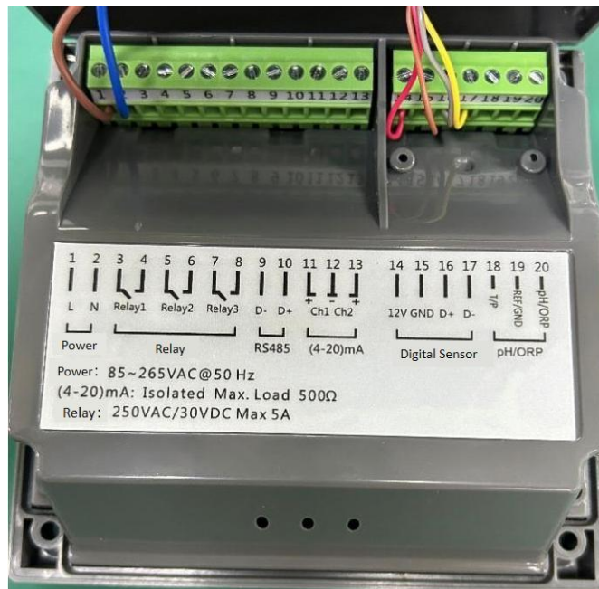
Figure 2-1 Controller Wiring Diagram
