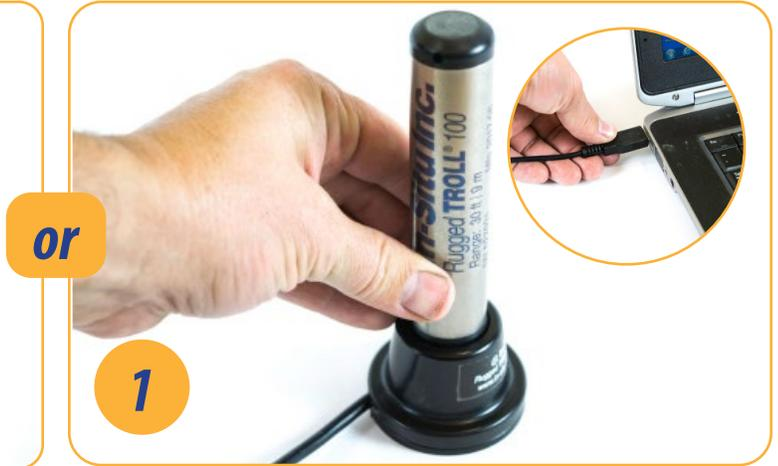
Connect the instrument to a computer and Win-Situ 5 software.
