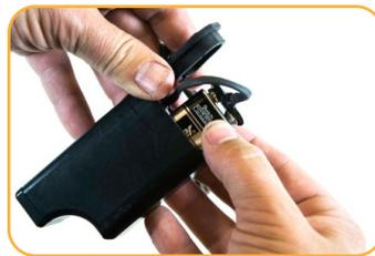
Attach the battery leads to the battery terminals.
