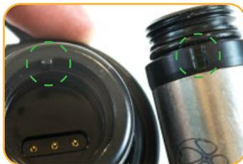
Invert the instrument. Align the notch on the instrument with the tab on the rim Rugged TROLL Cable. This will ensure that the pins are aligned to enable communication.
