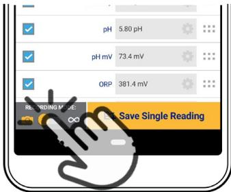
Tap the button on the bottom left to toggle between snapshot and live readings modes.
