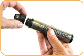
Unscrew and remove the hanger from the instrument.
