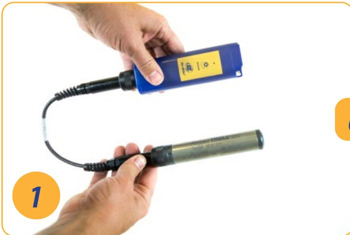
Attach the instrument to a Wireless Rugged TROLL Com and connect to the VuSitu mobile app.
