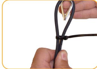
Place the metal loop inside the cable loop. Push the zip tie up to form a tight band around the metal loop.
