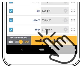
Tap **Start Recording**. The instrument takes a reading every two seconds.
