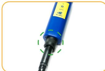
Connect the other end of the cable to the Wireless Rugged TROLL Com.
