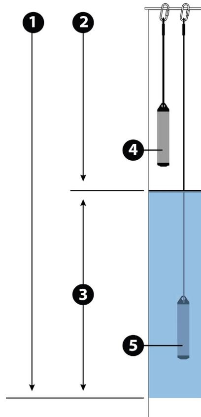
Figure 11.1 Rugged BaroTROLL and Rugged TROLL deployment
