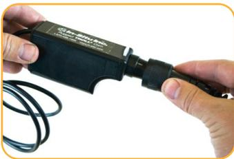
Attach the Rugged TROLL Com to the Rugged TROLL 200 cable via snap-on connection to the uphole end of the cable.
