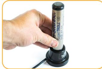
Place the instrument into the docking station.
