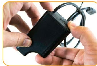
Push the battery into the compartment and close the door.
