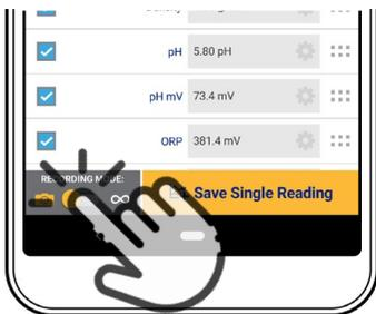
Tap the button on the bottom left to switch from snapshot mode to live readings mode.
