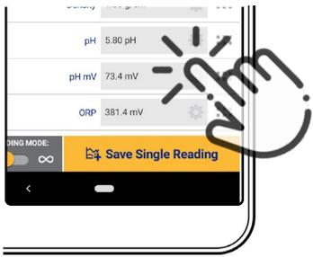
From the Live Readings screen, tap the settings wheel next to the field that contains the measurement value.
