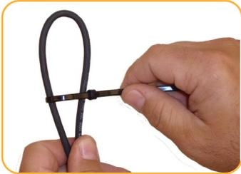
Create a loop on the uphole end of the cable and loosely bind it with one zip tie.
