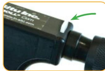
Release the connection to the uphole cable end by pushing in the white tab on the TROLL Com.
