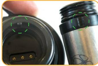
Invert the instrument. Align the notch on the instrument with the tab on the rim of the docking station. This will ensure that the pins are aligned to enable communication.
