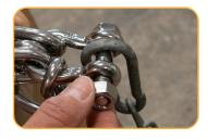
Remove cotter pin from anchor shackle. Unscrew bolt. Remove anchor or mooring point.
