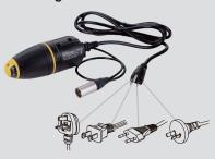
The Live Plug Connector (LPC separation filter) is used to safely inject a locate frequency onto a live street distribution cable using a standard household mains socket from a building. This allows the cable to be traced from the premises to the connection in the street.
