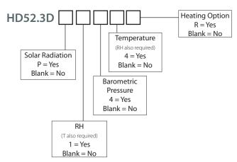
HD52.3D...: 2-axis ultrasonic static anemometer for the measurement of wind speed and direction, U-V Cartesian components of wind speed, Wind Gust, relative humidity and temperature (optional), global solar radiation (optional), barometric pressure (optional) and rainfall (optional). The "rainfall" and "global solar radiation" options are alternatives. Equipped with compass.
