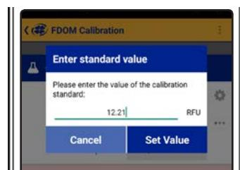
Enter the value shown on top of the calibrator into VuSitu. Press **Set Value**.
