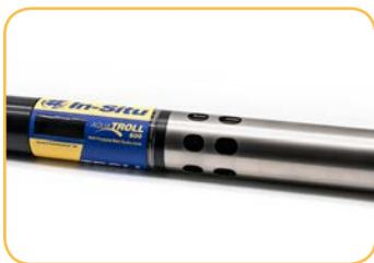
Put the Aqua TROLL restrictor in calibration mode. The holes should be near the center of the instrument.
