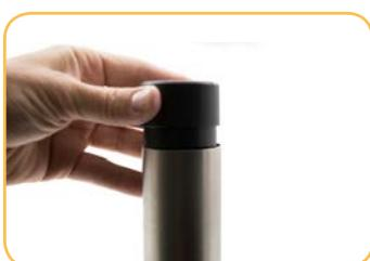
Place the solid state calibrator on the instrument as shown in VuSitu. Press **Next**.
