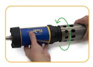
Install restrictor on the instrument.
