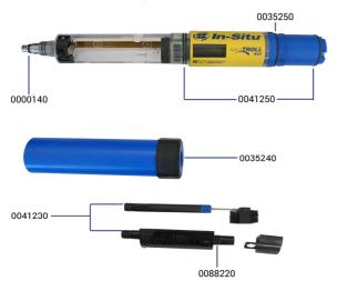
O-rings in the bag labeled 0041230 are used for all sensors, port plugs, and the wiper.
